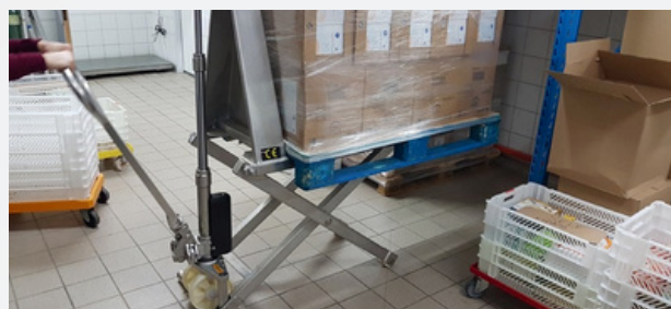
High lift manual pallet truck HAPPYPALIFT
